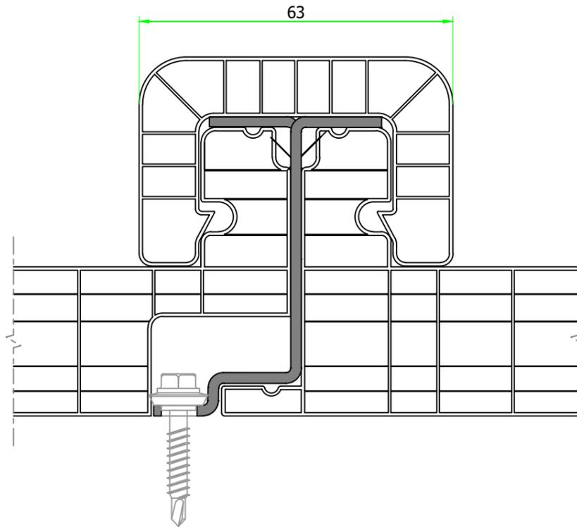
DETALLE DE ENCAJE MONTAJE LUCERNARIO CORRIDO **ESCALA 1:1**
